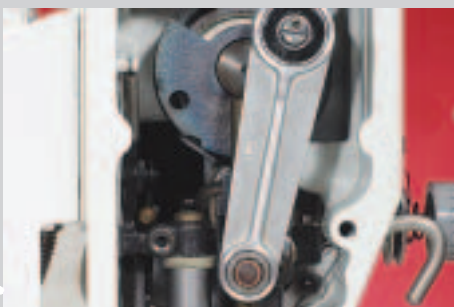
One machine for thick and thin material: adjustable needle bar stroke
