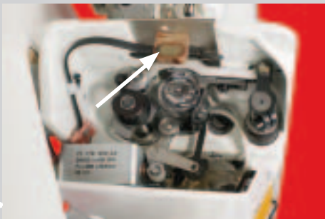
+ Bobbin thread monitor with rest thread sensor -926/06 (optional)
