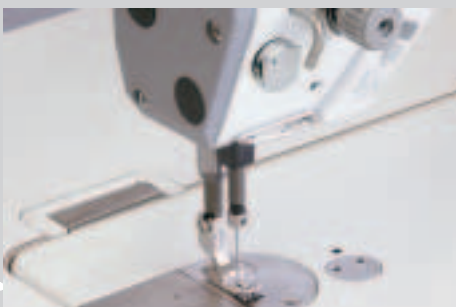
+ The new controlled thread nipper -909/14 always ensures a neat seam start
